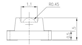
For reflow soldering (propose)
